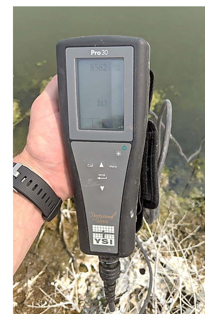
A YSI Pro30 handheld meter was used to measure specific conductance
